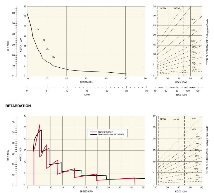
Instructions: From intersection of vehicle weight with percentage resistance line read across to determine maximum gear attainable, and then downwards for speed.
