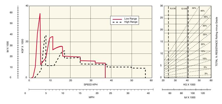
Instructions: From intersection of vehicle weight with percentage resistance line read across to determine maximum gear attainable, and then downwards for vehicle speed.
