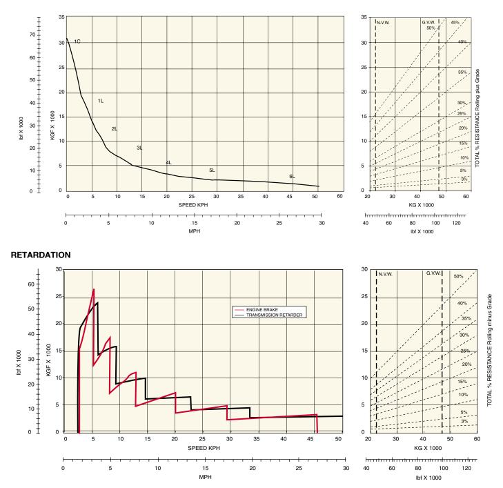
Instructions: From intersection of vehicle weight with percentage resistance line read across to determine maximum gear attainability, and then downwards for speed.
